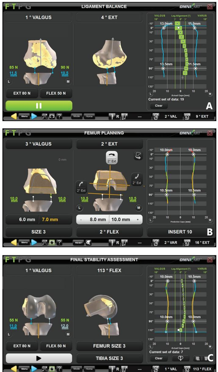
Fig 2. Screenshots from the OMNIBotics system showing (A) native gap balancing collection screen, (B) femoral planning screen and (C) implants gap acquisition screen
